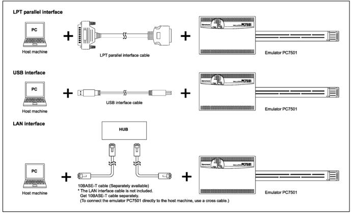
Figure 2.2 Outline for interface cable connections
